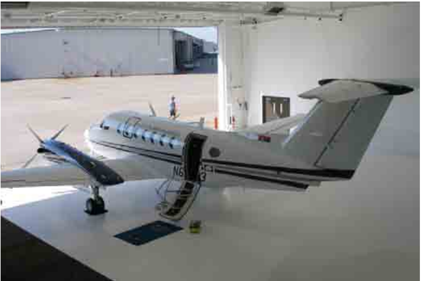
Figure 29. Aircraft “Hawker Beechcraft King Air 350” with an Integrated Flight Inspection System
